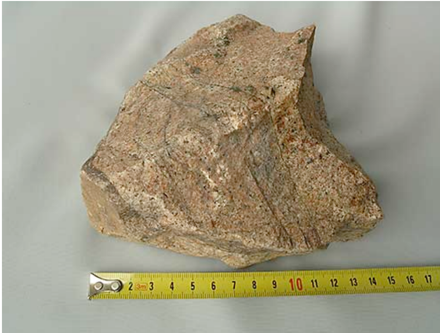
Fig. 21: In all directions cracked and quartz-cured granite (Pos. T)
