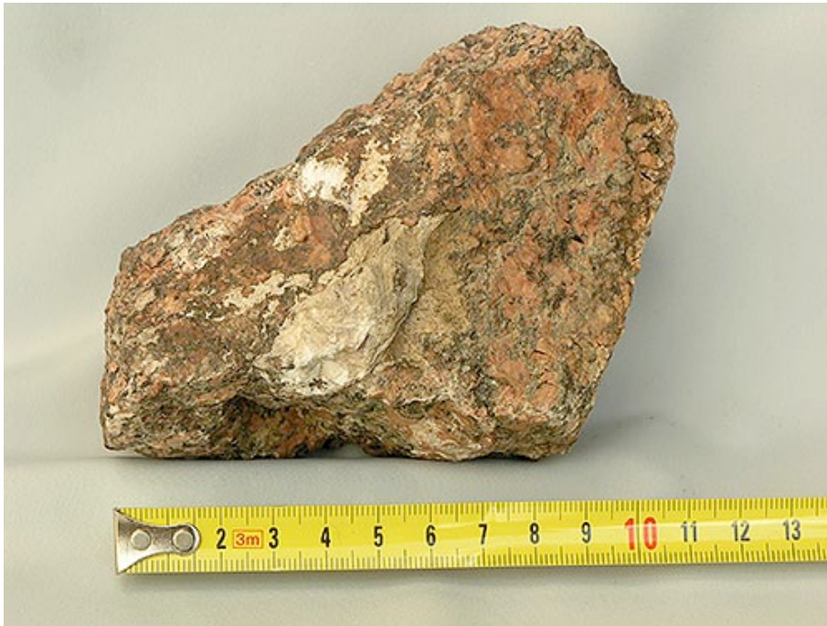
Fig. 16b: Mechanical calcite inclusions in reconstructed granite, Trolldalarna (Pos. Q).
