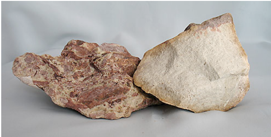
Fig. 34: Right part: Undamaged Silurian sandstone from nearby. Left part: Same sandstone after catastrophic event.
