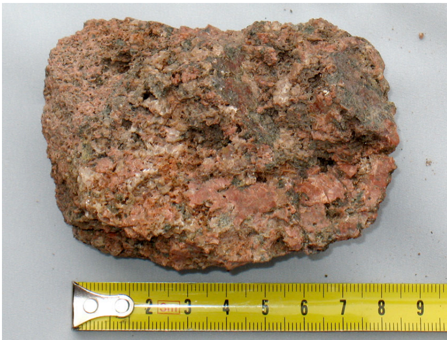
Fig. 8d: Highly porous sample of reconstructed granite.
