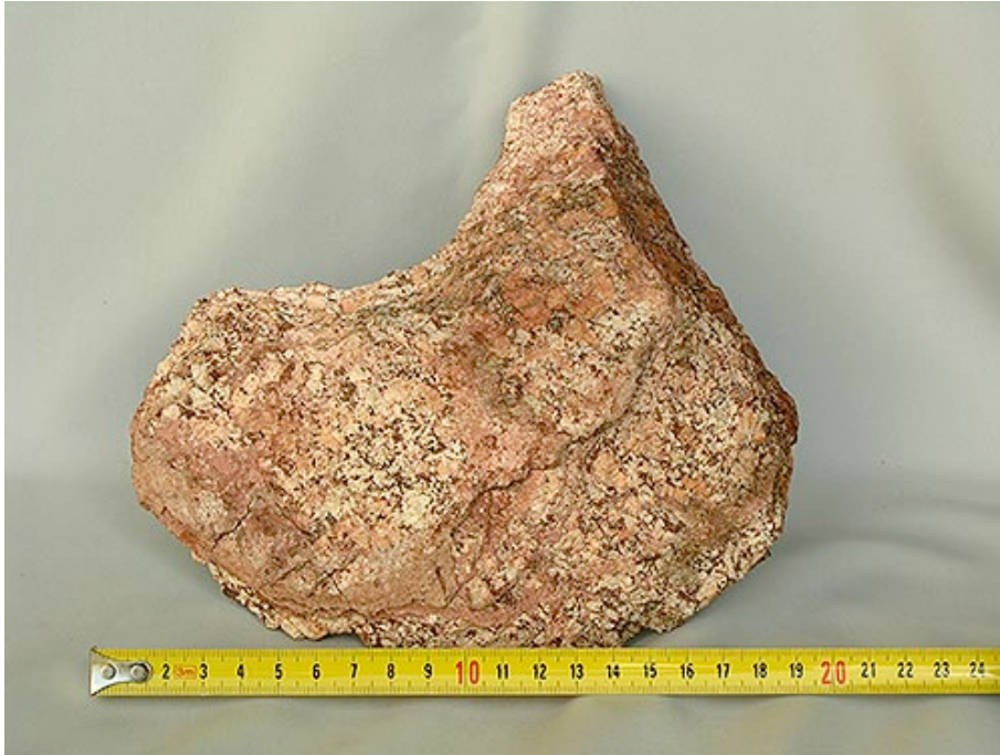
Fig. 30: Red-brown melt and reconstructed granite (Pos. Ap).
