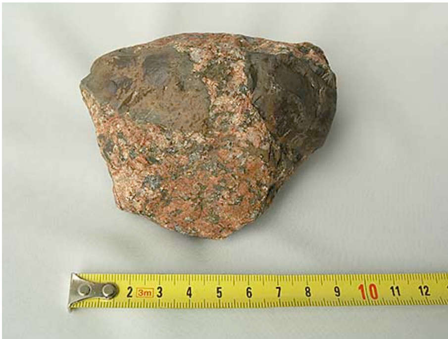
Fig. 16a: Egg-size drops of glass on reconstructed granite, Trolldalarna (Pos. Q).
