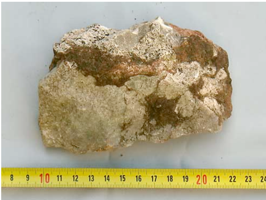
Fig. 43: Same sample as in fig. 42, but surface exposed to erosion. Pieces of reconstructed limestone separated from reconstructed Orsa sandstone
