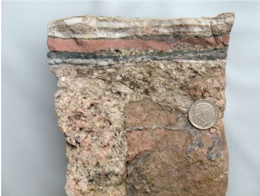
Fig. 33a: Melts of different melting point within the same sample. Coin 25 mm diameter.
