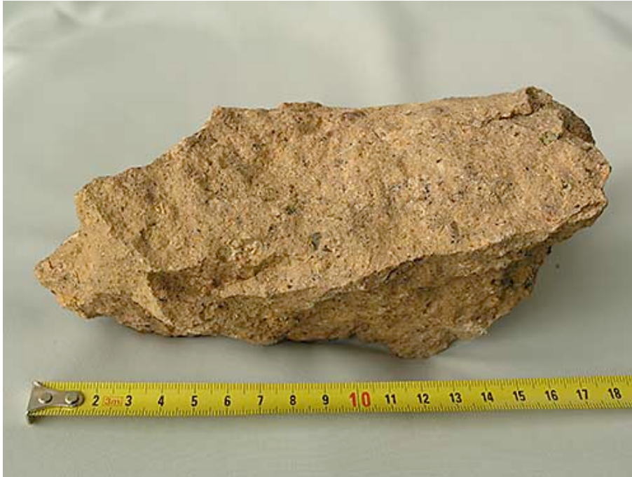
Fig. 7: The sample resembles sintered 'volcanic' ash (Pos. G).
