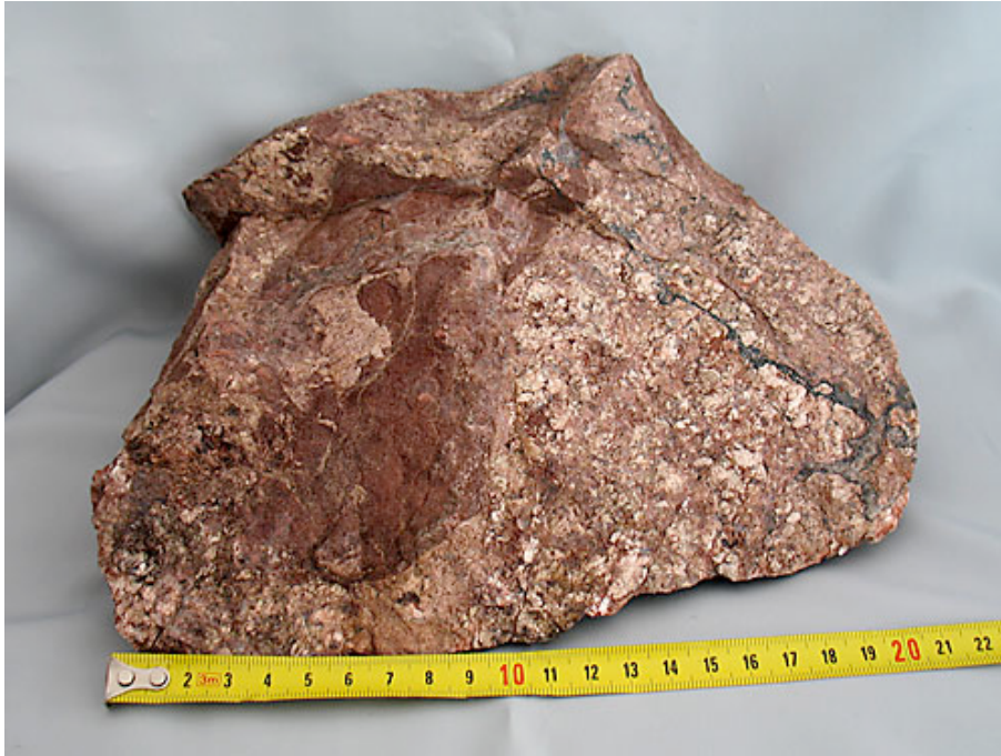
Fig. 31: Left part: Cracks in the solid roof, filled with melt. Right part: Dots of residual eutectic melt.
