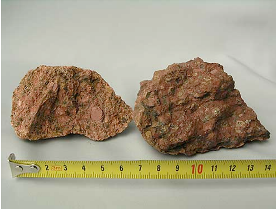
Fig. 13: Very dark red microcline like that formed from mylonite in a slip cracks. The dark dots are rounded grains of quartz.
