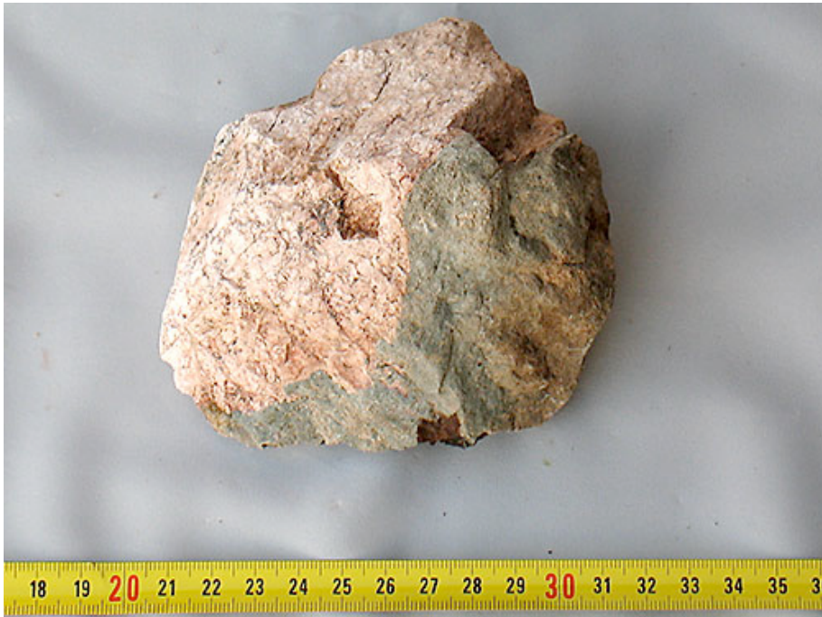
Fig. 32: Even blocks of dolerite, which happened to be at the site of impact, have been remelted and form a sharp zigzag border with the partly melted granite.
