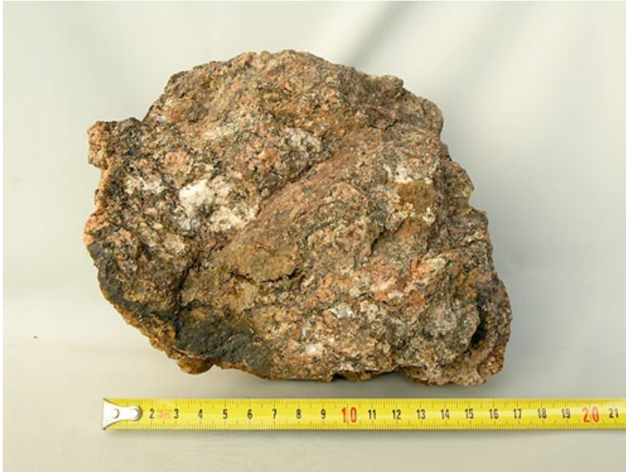
Fig. 8a: The sample contains a darker melt than that from Lake Siljan and some agglomerated calcite (Pos. H).
