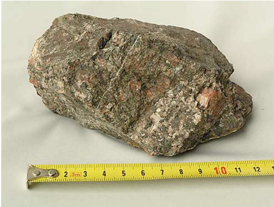
Fig. 9: Plenty of dark glass in this sample. The white dots are calcite and a calcium-silicate (Pos. N).
