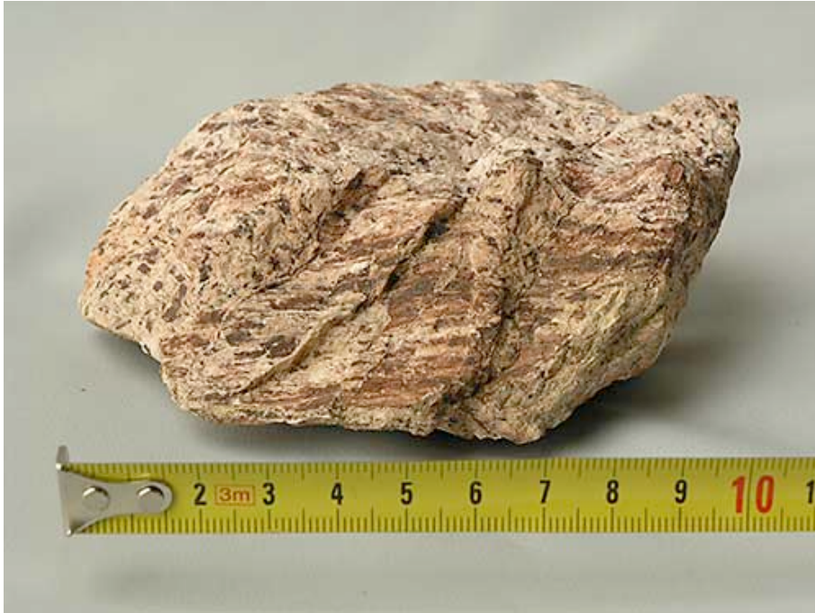
Fig. 3: Pseudotachylites in sheared granite (Pos. B).
