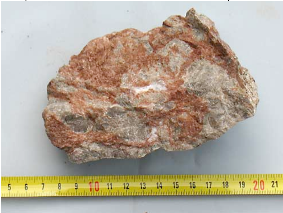
Fig. 42: Pieces of reconstructed brown Orsa sandstone and reconstructed grey limestone. The whole material has been pulverised during the impact. Fresh broken surface of same sample as in Fig. 43.
