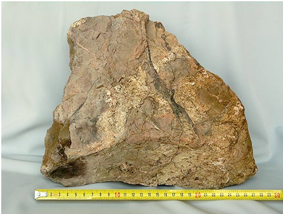
Fig. 29: Pink grey parts: Melt; light parts: Damaged original granite (Pos. Ap).
